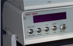
**PROGRAMMING** for three different device types may be entered into separate buffers. Each device wire may be programmed with individual ultrasonic power, time, and force (high or low) and loop elevation control data. Program values, action prompts, and fault diagnostics are exhibited on the easy to read 4 lines, 40 characters LCD sequentially with machine operation.
