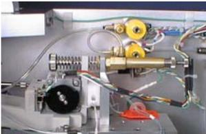
**FEATURES** include programmable dual force (high or low), bond tool positioning utility, and pneumatic braking of Z and Y-axes during bonding. Available with or without adjustable height platform.
