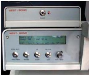
**PROGRAMMING** for thirty different device types may be entered into separate buffers. Each device wire may have up to 21 stitch bonds with individual ultrasonic power, time, force (high or low) and loop elevation control data. Program values, action prompts, and fault diagnostics are exhibited on the easy to read 4 line, 40 character LCD sequentially with machine operation.
