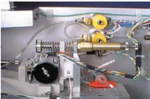
**FEATURES** include programmable dual force (high or low), bond tool positioning utility, pneumatic braking of Z and Y axes during bonding, and radiant tool heat. Available with or without adjustable height platform.
