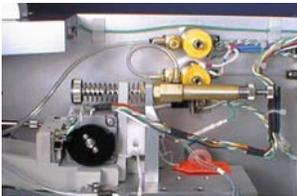
**FEATURES** include programmable dual force (high or low), bond tool positioning utility, and pneumatic braking of Z and Y-axes during bonding. Available with or without adjustable height platform.
