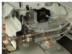
**PROGRAMMING** for thirty different device types may be entered into separate buffers. Each device wire may have up to 21 stitch bonds with individual ultrasonic power, time, force (high or low) and Z-Axes elevation control data. Program values, action prompts, and fault diagnostics are exhibited on the easy to read 4 lines, 40 characters LCD sequentially with machine operation.
