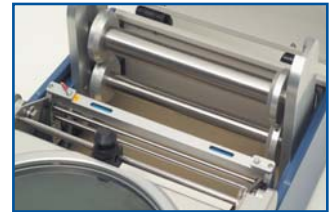
Automatic reeling and removal of UV tape backing
